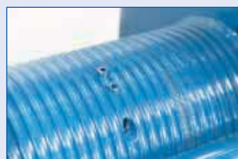
Additional rope anchor
