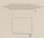
clouds. This electricity is generally positive. Let C in the figure represent a cloud charged with positive electricity. Let B represent a building on the earth beneath. The positive electricity of the cloud will attract the negative of the building and earth to the upper part of the building and will repel the positive away into the earth beneath.
