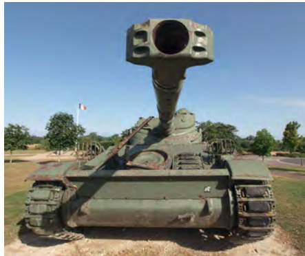
ABOVE: An AMX-13, also with a 90mm gun, at Monuments de Chars near Berry-aux-Bac, France. PHOTO COURTESY OF ALF VAN BEEM BELOW: Another shot of the AMX-13 exhibited along the Chemin des Dames, Aisne, France. The 90mm gun has a single baffle muzzle brake, while the 105mm weapon has a double baffle muzzle brake PHOTO COURTESY OF VASSIL
