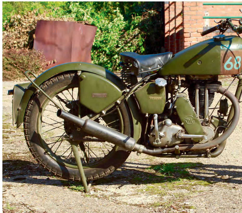
G3/L featured smaller bore exhaust and slimmed-down barrel finning, to save weight. But the dynamo was still a pain for REME workshops. Note wartime absence of rubber for pedals and controls.
