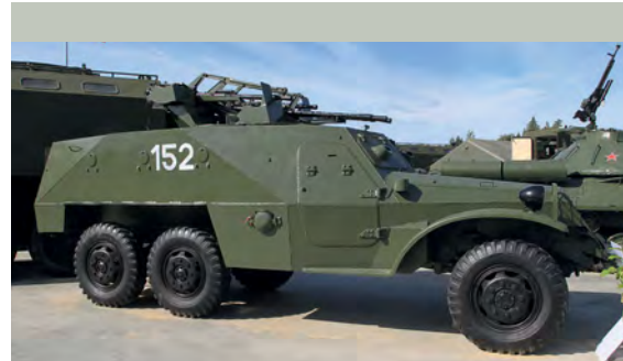
The BTR-152A, armed with the ZTPU-4 quad 14.5mm air defence system (ALEKSANDR KOSHAVTSEV)
