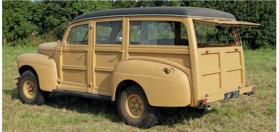
There were two different variants produced, a seven-seater and a five-seater like this example here. This model has the extra luggage compartment which can be accessed by lifting the rear window
