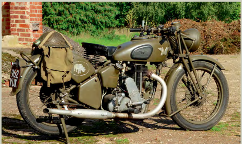
Despite weighty ancillaries, G3 WO was based on a pre-war sportster and originally gave livelier performance than lower compression G3/L
