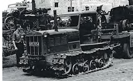
ABOVE: An STZ-3 in standard civilian configuration, with agricultural tracks, perhaps at the end of the war judging by the 'scrapyard' setting
