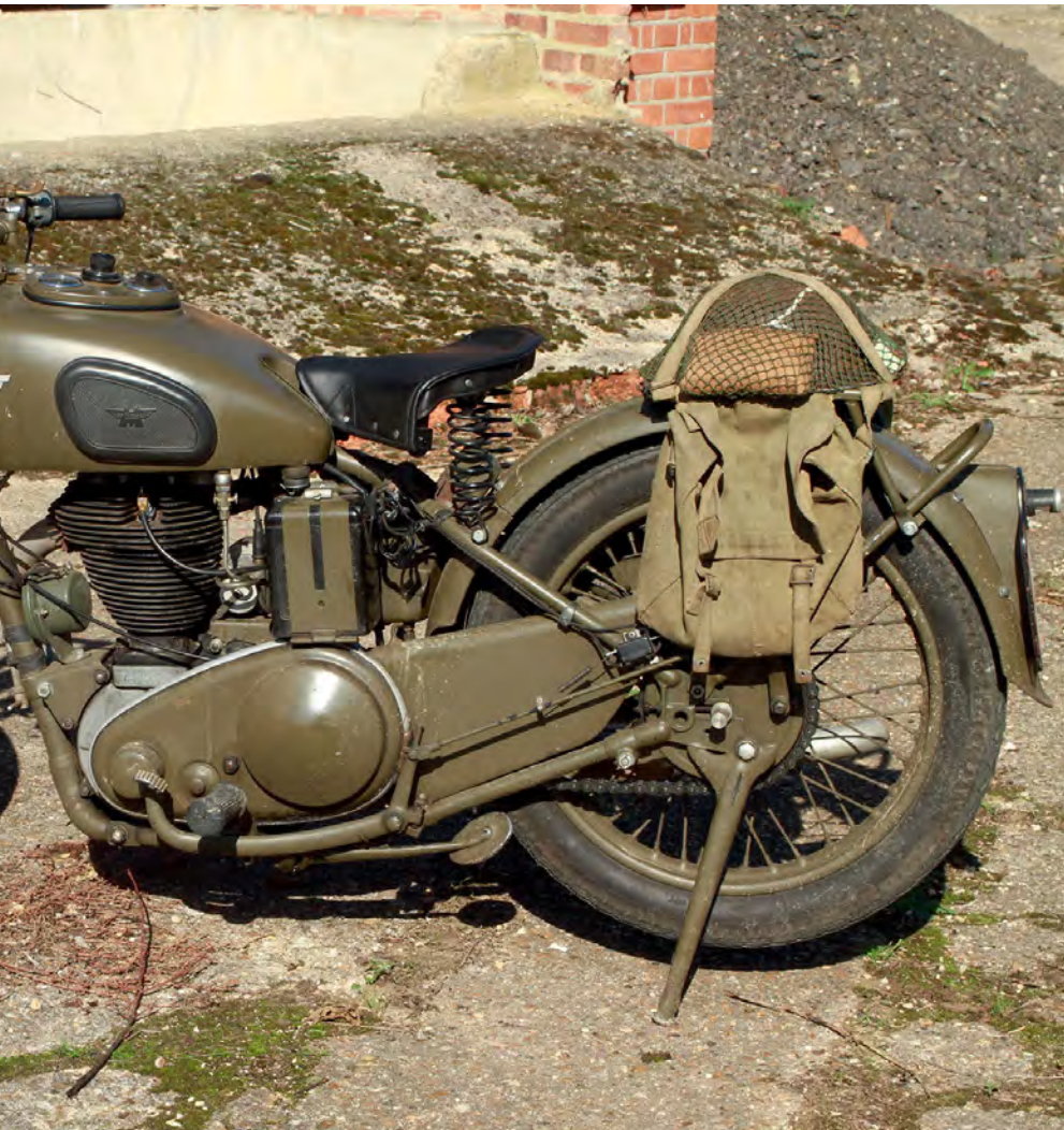
This early model G3 WO featured a prominent steering damper plus tank-top instruments, both dropped on the G3/L to save weight."
