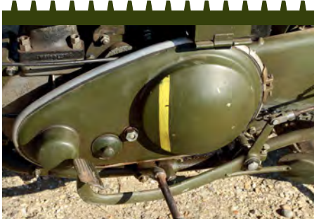
Yellow stripe on primary chaincase indicated centre of gravity, to help loading glider-borne machinery
