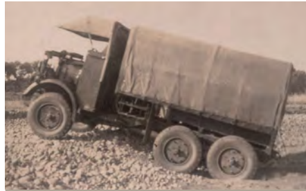
ABOVE: The 19.6hp Crossley climbs the loose rocks of No2 Obstacle on Chakala's testing ground BOTTOM: The No3 Obstacle comprised small stones and loose sand that would have sapped the Crossley's engine power BELOW: The Crossley light six-wheeler being driven on the loose going of Obstacle No4
