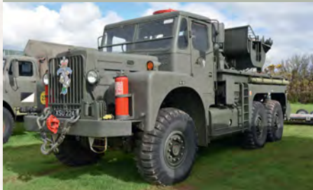
In this guise, the 1951 Leyland Martian is officially the 10-ton, 6x6, Heavy Recovery FV1119 truck and is Rolls Royce B81-powered
