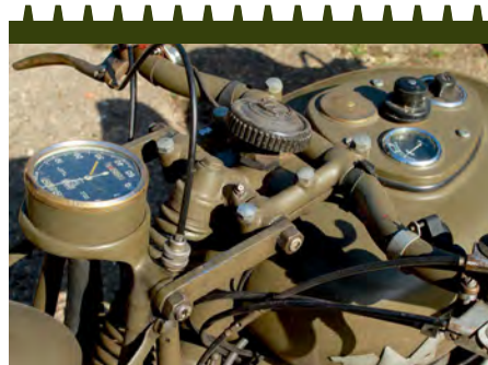
This early model G3 WO featured a prominent steering damper plus tank-top instruments, both dropped on the G3/L to save weight."
