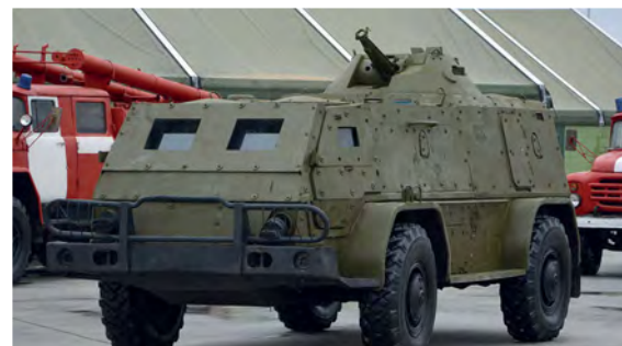
The GAZ-3937 'Vodnik' has now been in service for some years. This prototype is fitted with ceramic combination armour
