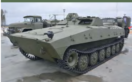
The RKhM chemical reconnaissance vehicle was almost unknown for most of its service life. It is based on the 2S1 self-propelled artillery vehicle
