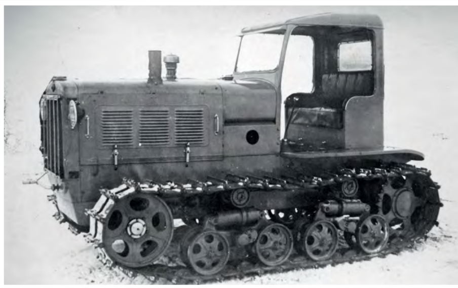
LEFT: The SKhTZ-NATI tracked agricultural tractor was produced at KhTZ in Kharkov. After the outbreak of war it was also used as an artillery tractor BELOW: An STZ-3 agricultural tractor destroyed while in use as an artillery tractor with the Red Army
