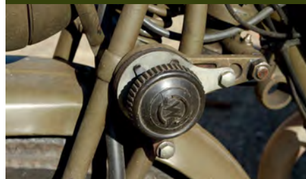
G3 WO's girder fork, featuring check-spring dampers, was fine of its type, but the G3/L's telescopic made it history
