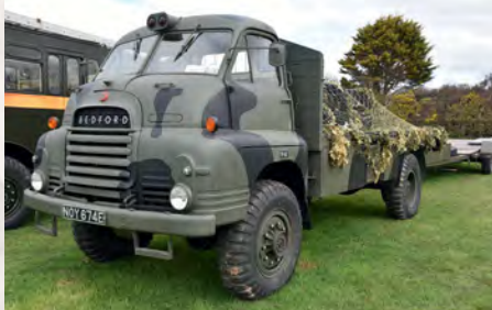
The three-ton, 4x4 Bedford RL was supplied in numerous variations, including air-portable, in the FV13000 series from 1952
