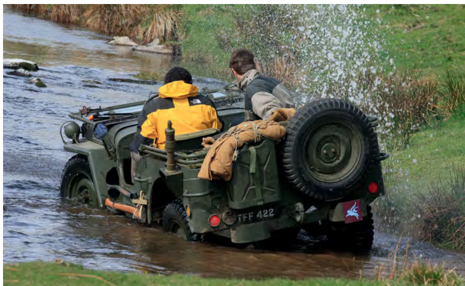
ABOVE: The Land of the Far Horizons BELOW LEFT: The beginning of the long climb to the border with Scotland BELOW RIGHT: This attempt to ford the river too quickly led to slipping into deeper water and a broken half shaft BOTTOM LEFT: A bright and chilly morning run through Stewartshiels Forest led by a Hotchkiss M201 BOTTOM RIGHT: In memory of Pilot Officer Martin Walter Rivers who died on April 25, 1941, age 24
