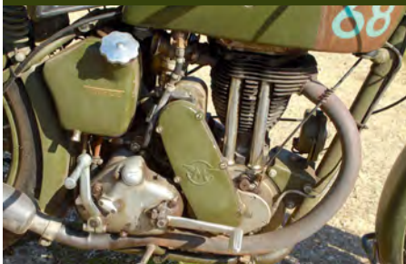
G3/L featured smaller bore exhaust and slimmed-down barrel finning, to save weight. But the dynamo was still a pain for REME workshops. Note wartime absence of rubber for pedals and controls.
