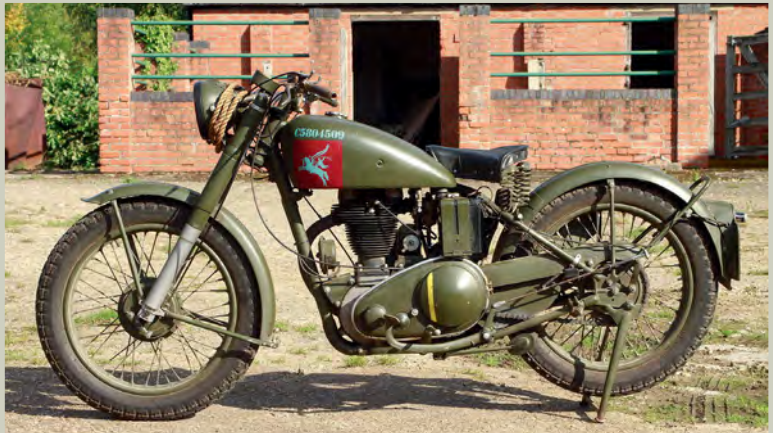
G3/L's light and eager looks were not deceptive. List of items changed on the prototype to get the weight down to 319 lbs ran to five pages
