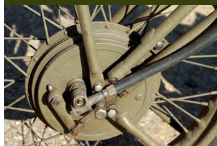
Many detail differences between this G3 WO and the G3/L included the former's bulkier rear chain guard, and front wheel drive for the speedo. A fine machine but with a foot in the past
