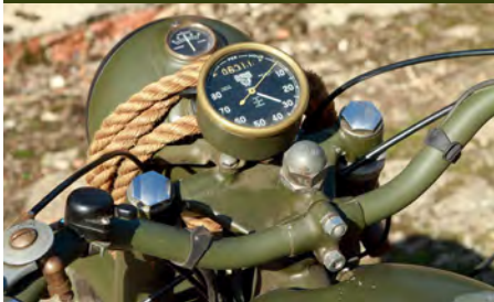
G3/L's separate speedo, no longer driven from the front wheel, and headlamp-mounted ammeter replacing early G3 WO's tank-top instruments.
