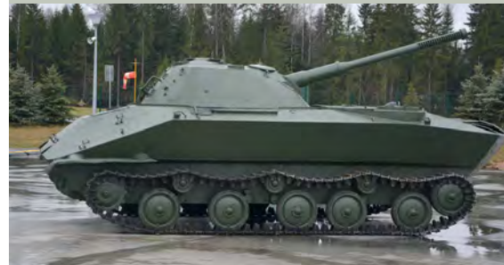
The K-90 amphibious light tank was developed on the chassis of the M2 artillery tractor. It was the predecessor to the PT-76
