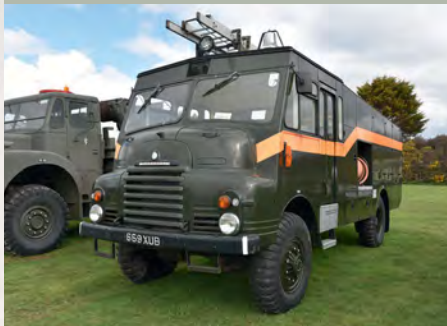
THIS 1960 Green Goddess is a fire engine variant of the three-ton Bedford designated RLHZ built to Home Office specification and used mainly by Auxilliary Fire Service units
