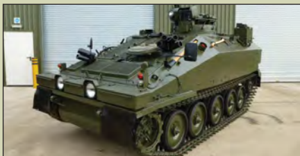
Spartan CVRT Dieselised APC , Fitted Cummins BTA 5.9lt Turbo diesel engine, Engine: power 195 hp, David Brown TN15d Epicyclic Semi-Automatic Gearbox with Neutral turn capability, Max road speed 72 km/h, Range 750 km, Manoeuvrability, Gradient 60%, Side slope 35%, Vertical step 0.5 m, Trench 2m, Fording 1m etc, Ex condition, ..... Guide price from £19,995 (3 Available)
