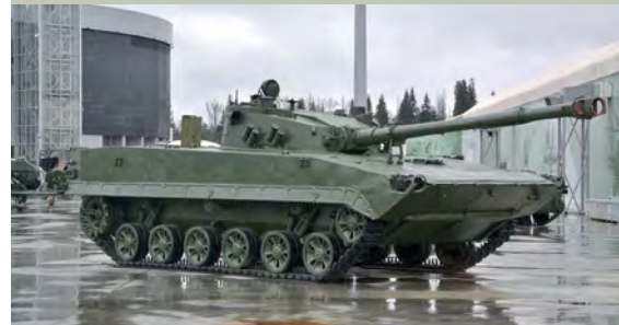
The Obiekt-685 was a potential replacement for the original BMP series. Armed with a 100mm 2A48 gun. It was one of the early prototypes for the current BMP-3
