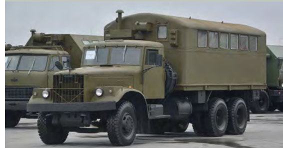
Many vehicles from the former Ryazan Military Vehicle Museum are now located at Patriot Park. Seen here a 6x4 KrAZ-219 MM4 maintenance vehicle
