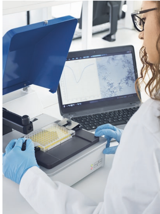
Fig. 1 Photograph of the open oCelloScope loaded with a 96-well plate. The UniExplorer software allows setting the experiment as well as performing online and offline image analysis along with generation of time-lapse videos. Growth/growth inhibition curves can be inspected and compared among the different wells
