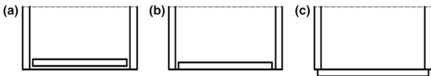
Fig. 2.22 Ways of inserting the fronts of drawers and doors to the body of the furniture piece: a inserting, b harmonising, c applying on
