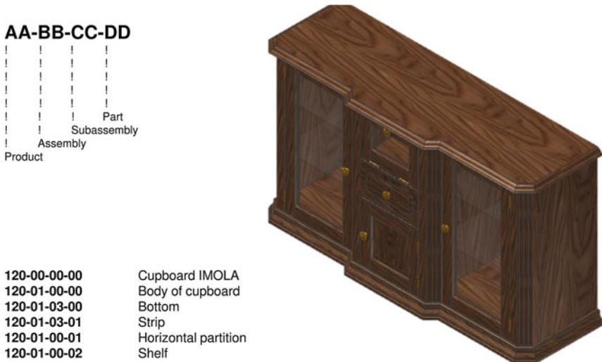
Fig. 5.5 An example of numbering drawings of a furniture piece, an assemblage, a subassemblage and element
