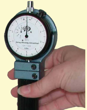
DBL-300 Shown being set with DBM- 1000 master
