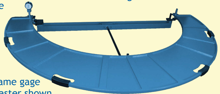
LD - Swing gage, where the heads rotate in for long retraction
