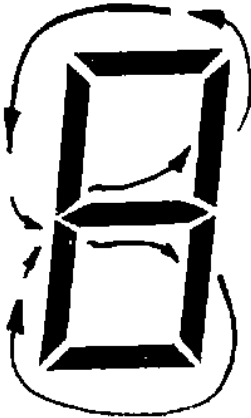
The LED turn-on sequence around the display.
