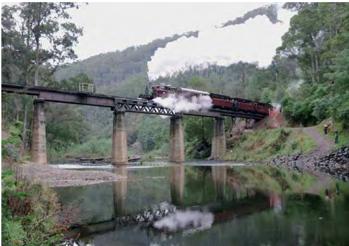
On Saturday 29 May, Puffing Billy's NA class 2-6-2T 7A (temporarily renumbered 9A for historical purposes) departs Thomson and crosses the Thomson River bridge with drain cocks open in preparation for the 1 in 30 grades ahead. Photo: Scott Gould
