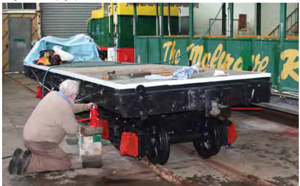
The overhaul and rebuild of a former Queensland Railways Innisfail Tramway 610mm gauge HHB wagon, obtained from Mourilyan Sugar Mill, is nearing completion in a Melbourne workshop. It is planned for utilise the rebuilt vehicle as a heavy-duty flat car.
