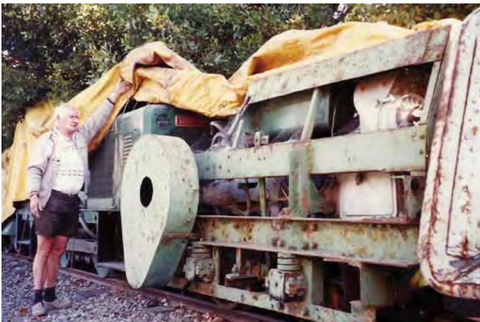
National Railway Museum's stalwart Ron Fluck lifts the tarpaulin to show two of the stored ex-Stenhouse Bay 610mm gauge locomotives, the rebuilt Malcolm Moore 4wDM with a Deutz engine (in the foreground) and Ruston & Hornsby 4wDM 306 (393981 of 1956) on 16 April 1998. Photo: Bob McKillop
