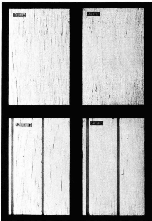
Figure 1—Typical differences between all-acrylic paint system No. 1 and alkyd-primed system No. 9 after exposure for 5.5 years in Tacoma. Finish No. 9 is shown in the left-hand photographs
