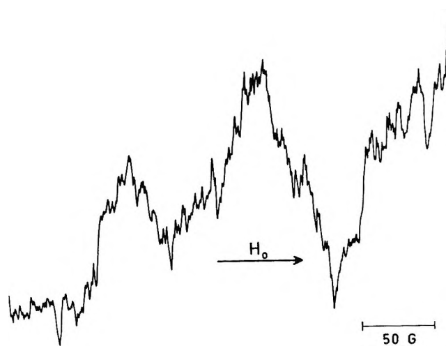
Figure 4. Epr spectrum of chloroformic solution of \text{Cu}(\text{BADO})_2 (at -160^\circ ).
