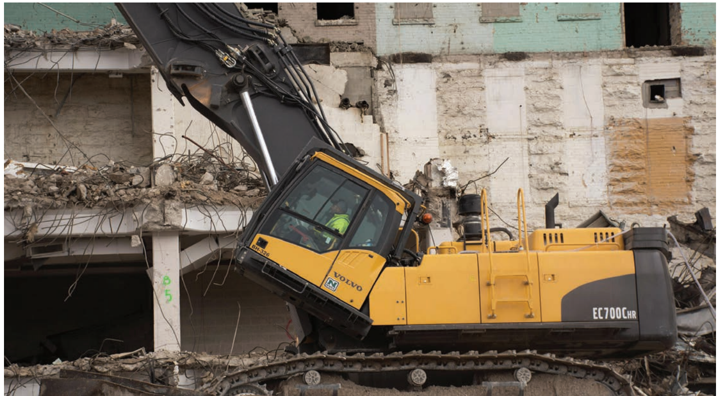
The 30° tilt offered by the Volvo cab increases operator visibility and comfort.
