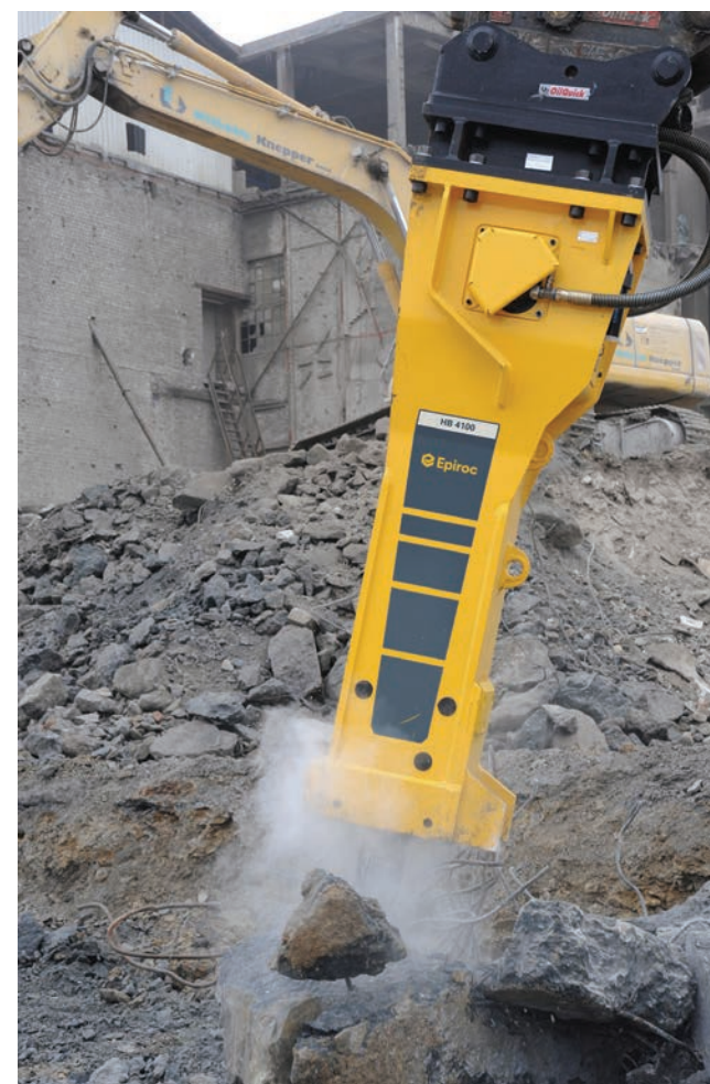
The system permits more accurate and significantly faster positioning of the breaker thanks to the centering effect, and avoids blank firing that often results in tool damage.
