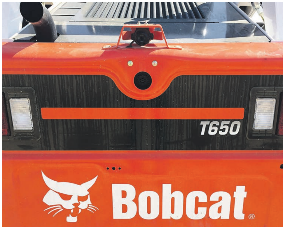
The system is integrated into the loader, activated when the ignition is turned on, and runs continuously as the loader moves in both forward and reverse motions.
