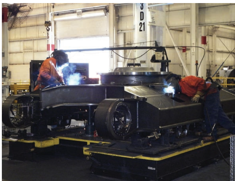
Welders work on an excavator track frame in the fabrication plant.
