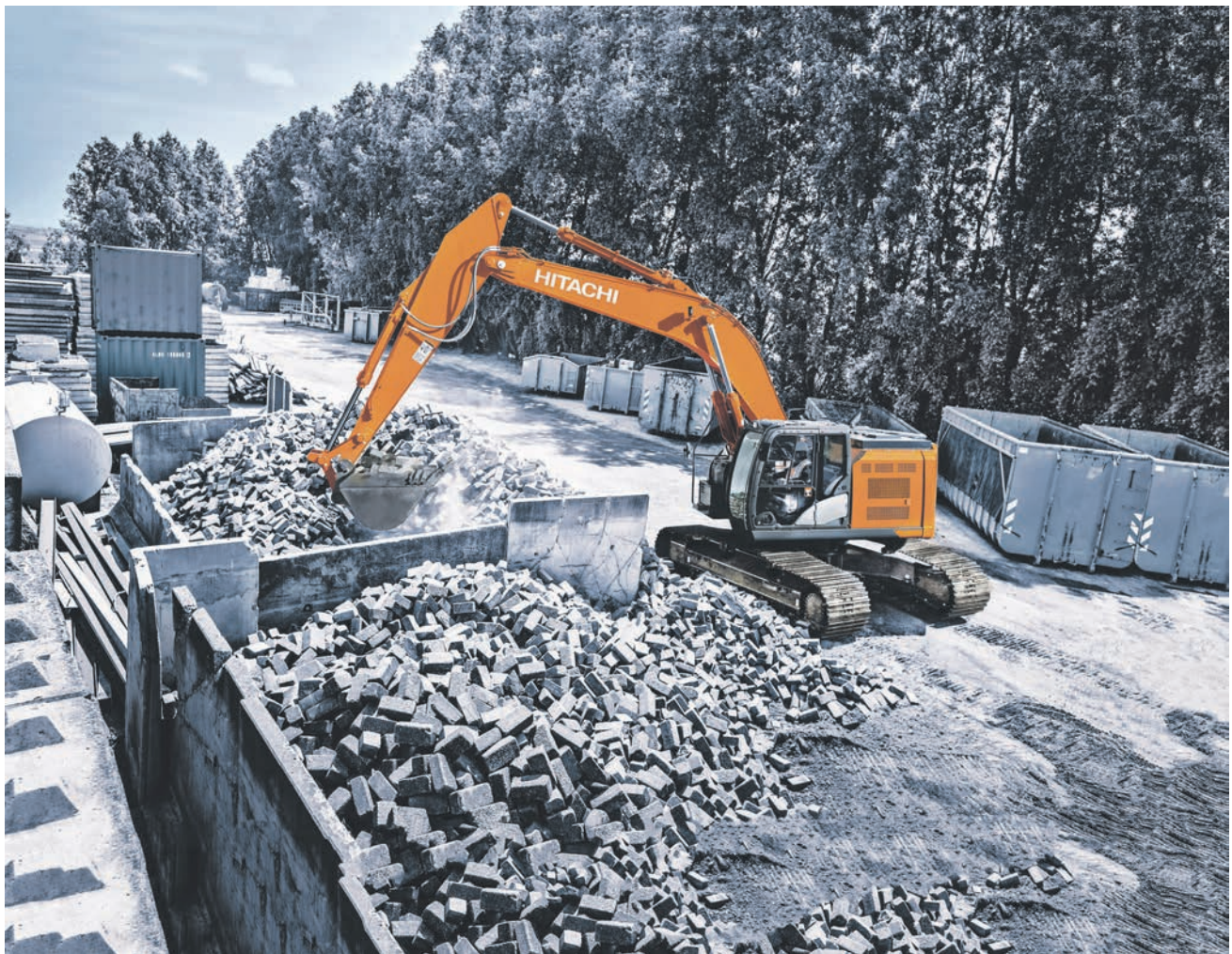
The heavy-duty undercarriage, designed for a 35-metric-ton machine, provides a low center of gravity, greater stability and increased lift capacity.
