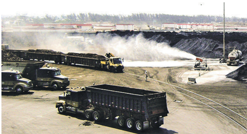
Atomized mist creates a wide area of airborne and surface dust control at the point of emission.
