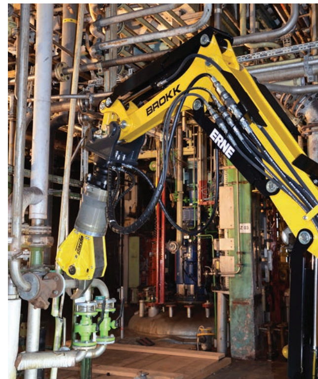
The small Brokk 100, 120 D and 160 remote-controlled demolition machines can use the lightweight Darda MC200 Multi Cutter steel cutting attachment to cut a variety of steel material in industries such as demolition, recycling, nuclear, process, food and construction.
