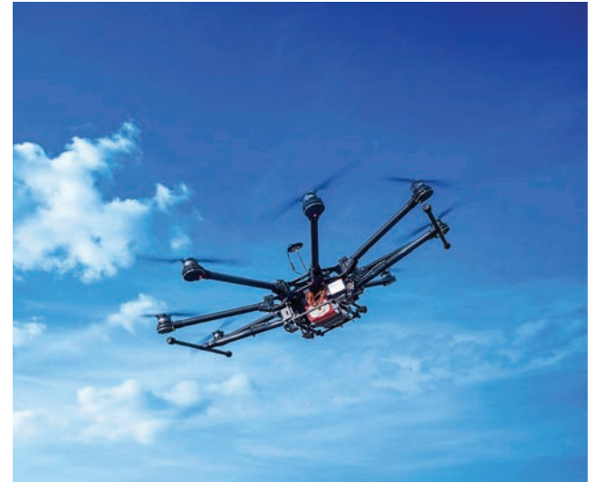
Drones can capture survey imagery, contribute to jobsite safety, provide time-lapse imagery and even thermal imaging to evaluate building envelopes and enclosures.
