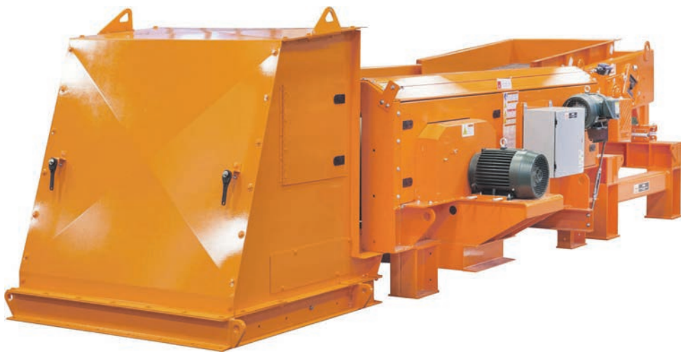
Introduced in 2016, the Eriez UHF Eddy Current Separator generates significant new revenue for scrap metal processors by recovering valuable aluminum, copper and other nonferrous fines.
