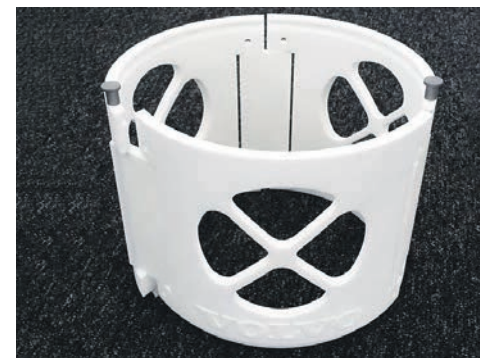
A workshop tool for mounting parts on an axle has been made by 3D printing.
