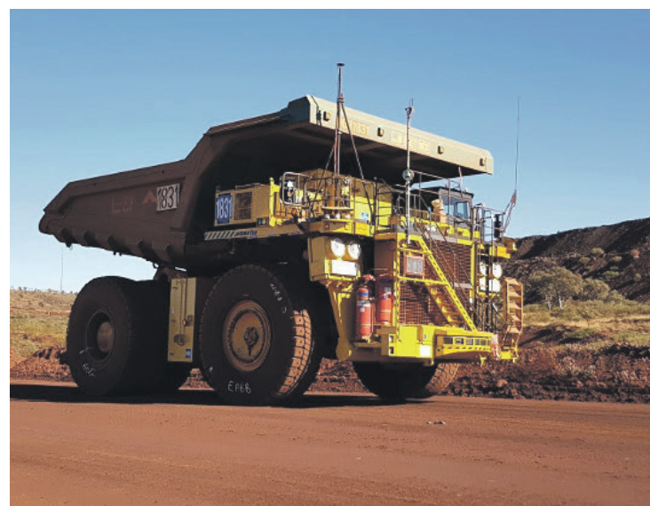
A standard truck 830E with the AHS retrofit kit running in autonomous mode at Rio Tinto's mine in Australia.
