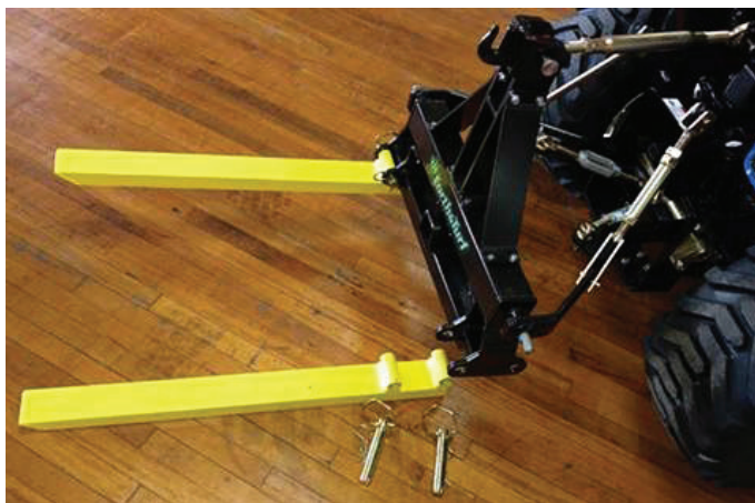
The tines are attached by lynch pins so they are both completely removable and can pivot upward for space-saving storage.
