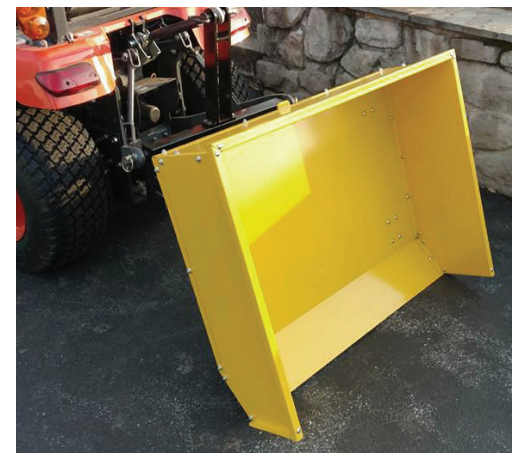
The cart has a weight capacity of 800 lbs and can be moved easily on smooth surfaces either empty or with a load.
