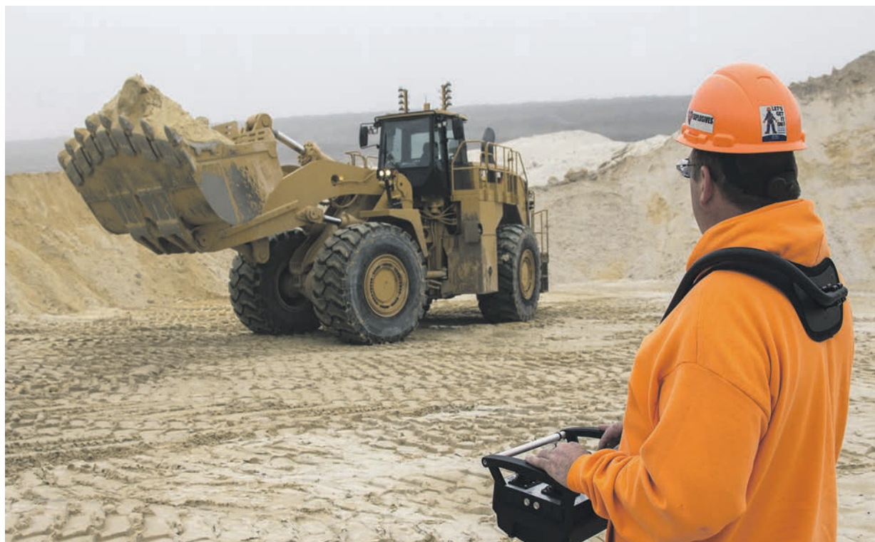
Cat® Command for loading reduces the risk of injury and enables production to continue by allowing safe operation of the loader in potentially hazardous environments.
