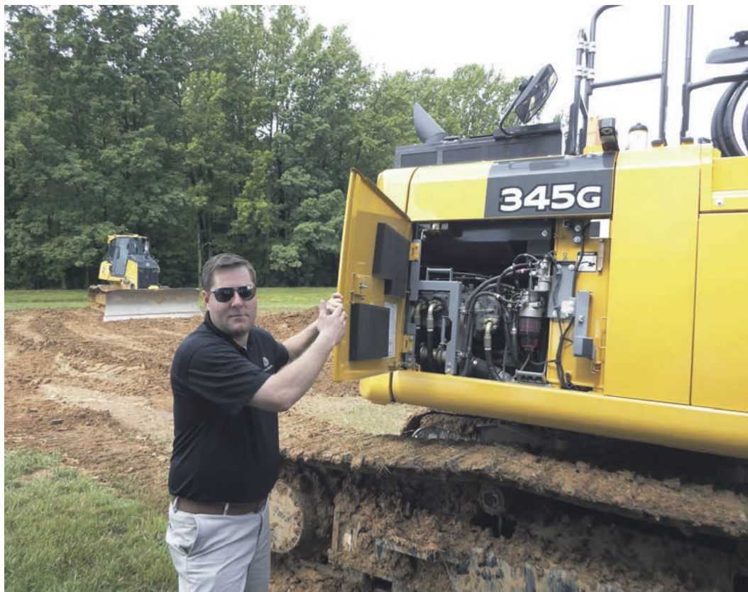
The 345C features three hydraulic pumps that provide optimum hydraulic pressure to various functions of the excavator when the demand is needed. Alex Anhalt, product consultant for excavators, explains how the systems work.
