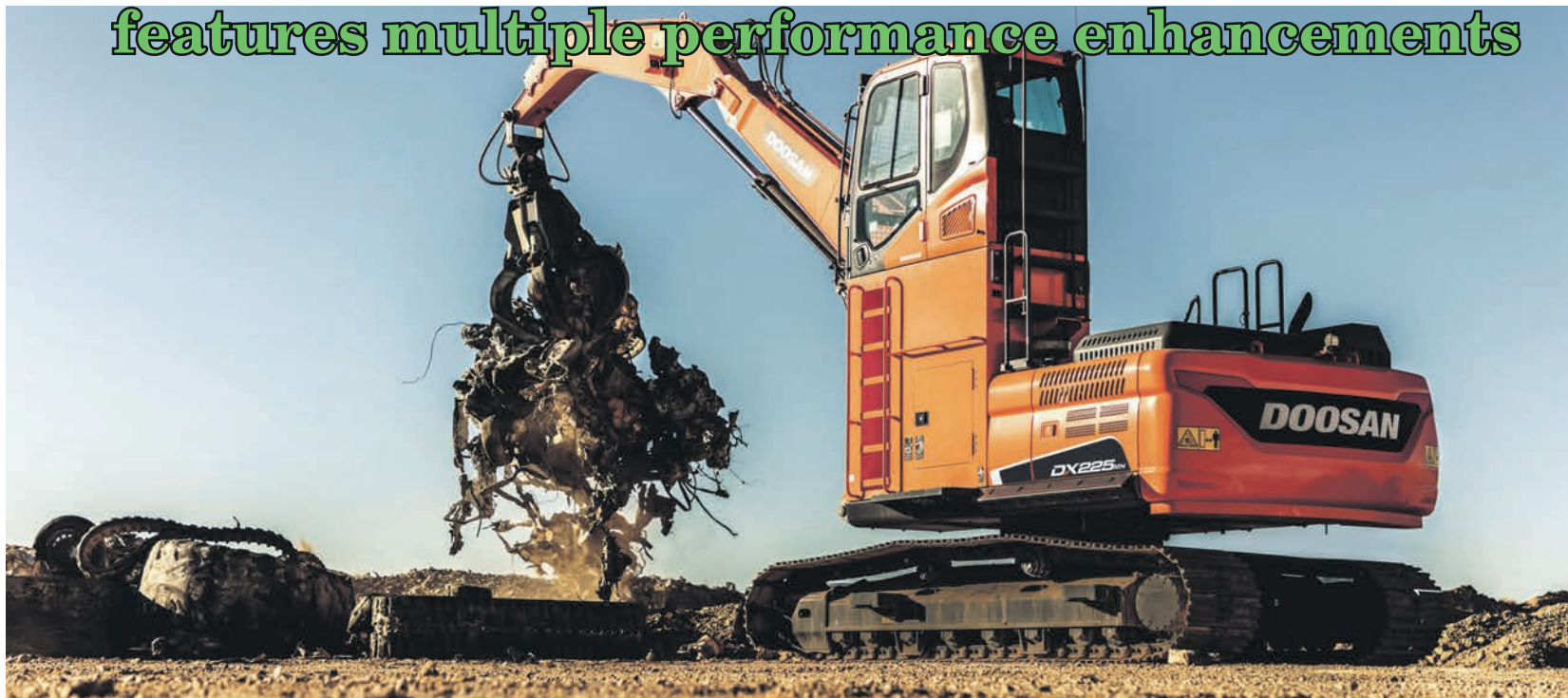
Machine features such as dual-boom cylinders and under-mount arm cylinder placement provide excellent lifting capabilities for Doosan material handler operators.
