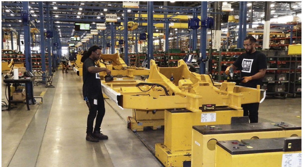
In the assembly plant, workers begin the assembly process by installing wiring harnesses into the excavator's mainframe.
