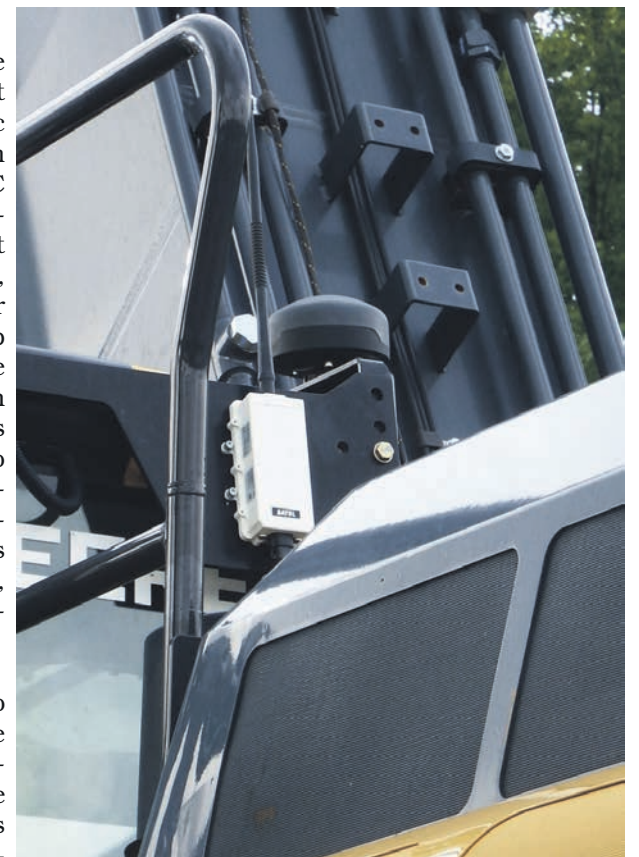
GPS telemetry enables the John Deere Excavator Grade Control System to perform at a high level of accuracy.
