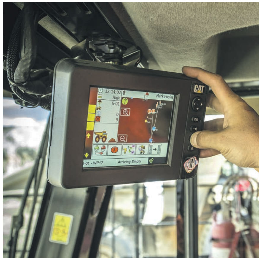
While Cat MineStar has always had a blending element, the new Blending to Destination feature expands blending capabilities to include wheel loaders and load-haul-dump scenarios.
