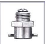
CCA-31300 Thread Size - 9/16" - 18 NF3 Brass, Cadmium Plated Length - 1.234" Lock Wire Drilled Action - Push to Open, Non-Lock Open
