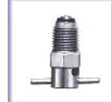
CCA-1600 Thread Size - 1/4" NPT Brass Length - 1.690" Action - Push to Open, Turn to Lock Open
