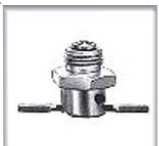
CCB-36650 Thread Size - 9/16" - 18 UNF-3A Brass, Cadmium Plated Length - 1.234" Lock Wire Drilled Action - Spiral, Non-Lock Open Not Recommended for fuel or oil
