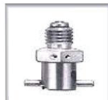
CCA-5800-1 Thread Size - 7/16" - 20 NF3 Brass, Cadmium Plated Length - 1.205" Lock Wire Drilled Action - Spiral, Non-Lock Open
