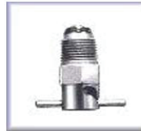
CCA-1350 Thread Size - 3/8" NPT Brass Length - 1.920" Action - Spiral, Lock Open
