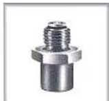
CCA-5800-3 Thread Size - 7/16" - 20 NF3 Brass, Cadmium Plated Length - 1.205" Lock Wire Drilled Action - Push to Open, Non-Lock Open
