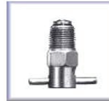
CCA-1550 Thread Size - 1/8" NPT Brass Length - 1.358" Action - Push to Open, Turn to Lock Open
