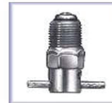
CCA-36150 Thread Size - 1/8" NPT Brass, Cadmium Plated Length - 1.358" Action - Spiral, Non-Lock Open
