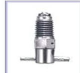
CCA-4800 Thread Size - 1/4" NPT Brass, Cadmium Plated Length - 1.690" Lock Wire Drilled Action - Push to Open, Turn to Lock Open
