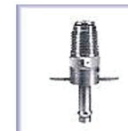
CCB-37000 Thread Size - 1/2" NPT Brass Body Length - 2.128" Stem Length - 1.125" Lock Wire Drilled Action - Push To Open, Turn To Lock Open
