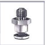
CCB-4320 Thread Size - 7/16" - 20 NF3 Brass, Cadmium Plated Length - 1.187" Lock Wire Drilled Action - Push to Open
