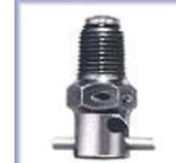
CCB-36750 Thread Size - 1/8" NPT Stainless Steel (303) Length - 1.358" Lock Wire Drilled Action - Spiral, Lock Open
