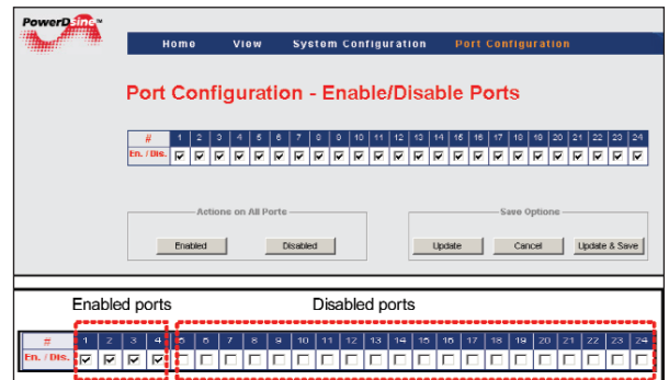
Port Configuration Enable/Disable. Each port may be individually enabled/disabled, or all ports may be enabled/disabled in one action.
