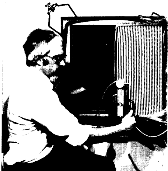
FIGURE 8: Mounting frame for HEPA filter with filter seat test groove
