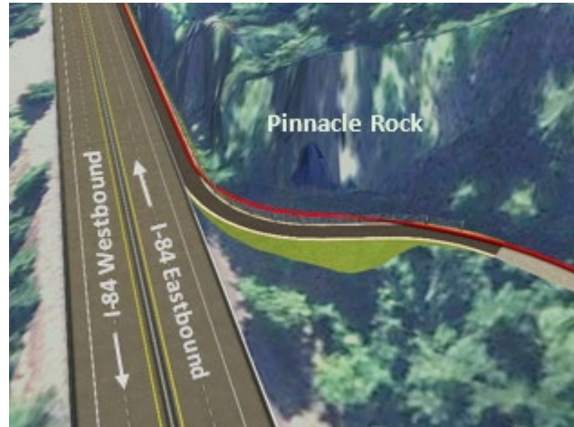
Figure 33: Trail Refinement at Pinnacle Rock West End (STA 348+00) with alternative alignment consider shown in red.
