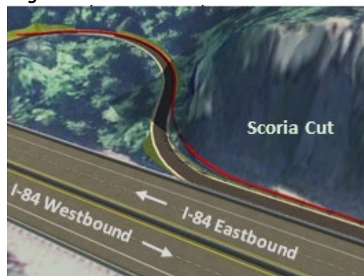
Figure 29: Trail Refinement at Scoria Cut East End (STA 334+00) with alternative alignment consider shown in red.
