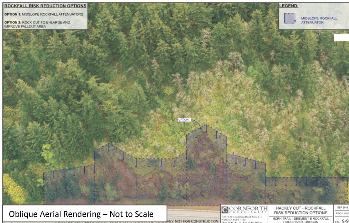
Figure 56: Hackley Cut Rockfall Risk Reduction Options
