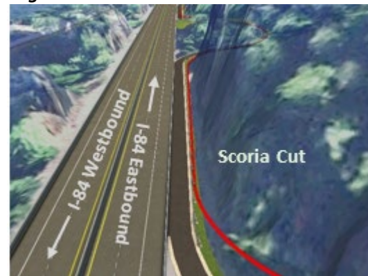
Figure 30: Trail Refinement at Scoria Cut (STA 332+00) with alternative alignment consider shown in red.
