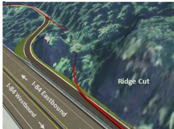
Figure 31: Trail Refinement at Ridge Cut East End (STA 343+00) with alternative alignment consider shown in red.
