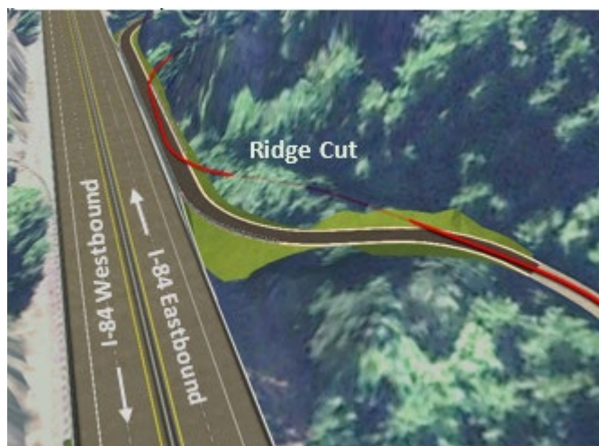
Figure 32: Trail Refinement at Ridge Cut West End (STA 339+00) with alternative alignment consider shown in red.
