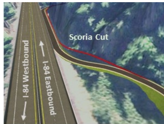
Figure 28: Trail Refinement at Scoria Cut West End (STA 329+00) with alternative alignment consider shown in red.
