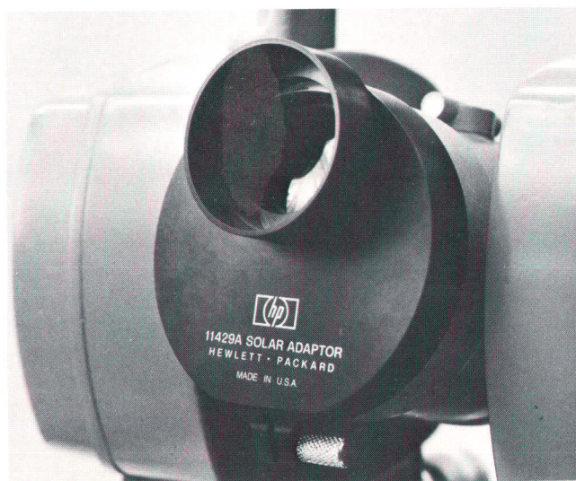
Fig. 3. Roelof's Solar Prism Adapter. This accessory for the 3820A allows measurement of the angle of the sun above the horizon.
