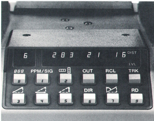
Fig. 4. Close-up view of 3820A keyboard and display. There are two of these units, one on each side of the instrument, for user convenience.
