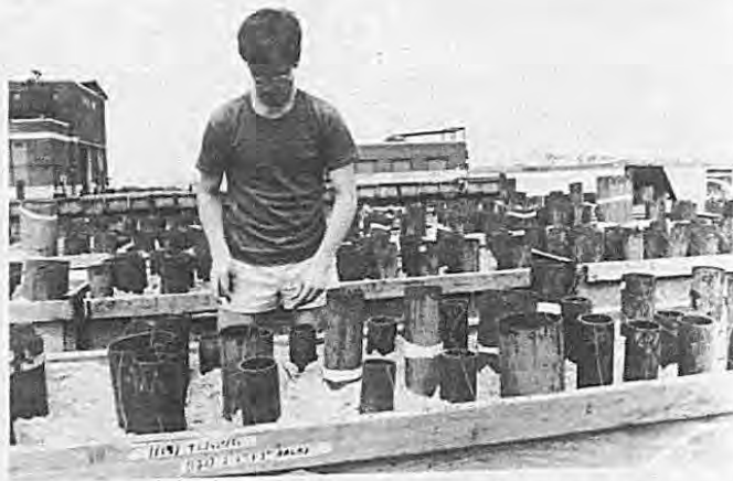
SETTING UP THE BATTERIES, Phil Grucci coordinates the display of fireworks for a waterside display. Each eight foot battery contains 1-1/2 tons of sand. The shells, placed in firing order, are set into firmly placed iron and steel mortars.
