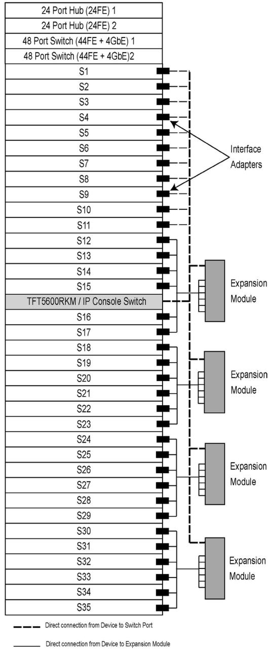
Figure 12 illustrates a maximum flexibility Ethernet cabling diagram.
