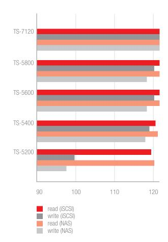
**Test environment:** N-Tec Rackmount Server Windows Server 2008R2, Dual XEON 32 GB RAM, 2 x IntelPRO/1000Dual = 4 x Gigabit NIC; Cisco SG300-10P 10 Port managed Gigabit with PoE.
