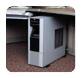
The HP 220mx offers 70 percent more capacity than its predecessor, the HP 125ex. With one or two multifunction 9.1 gb drives, 24 slots and a 12-second cartridge exchange time, it's a cost-effective entry to the HP jukebox family.
