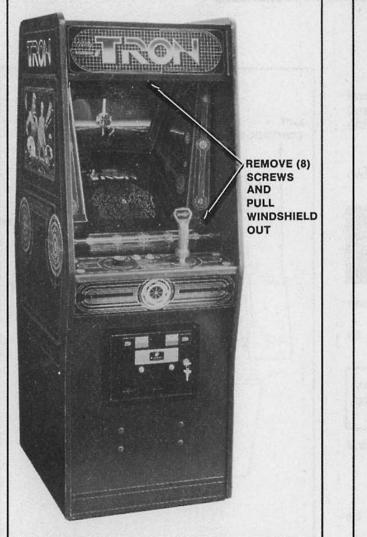
Figure 4-5 Removing Windshield & Windshield Retainers — Upright
