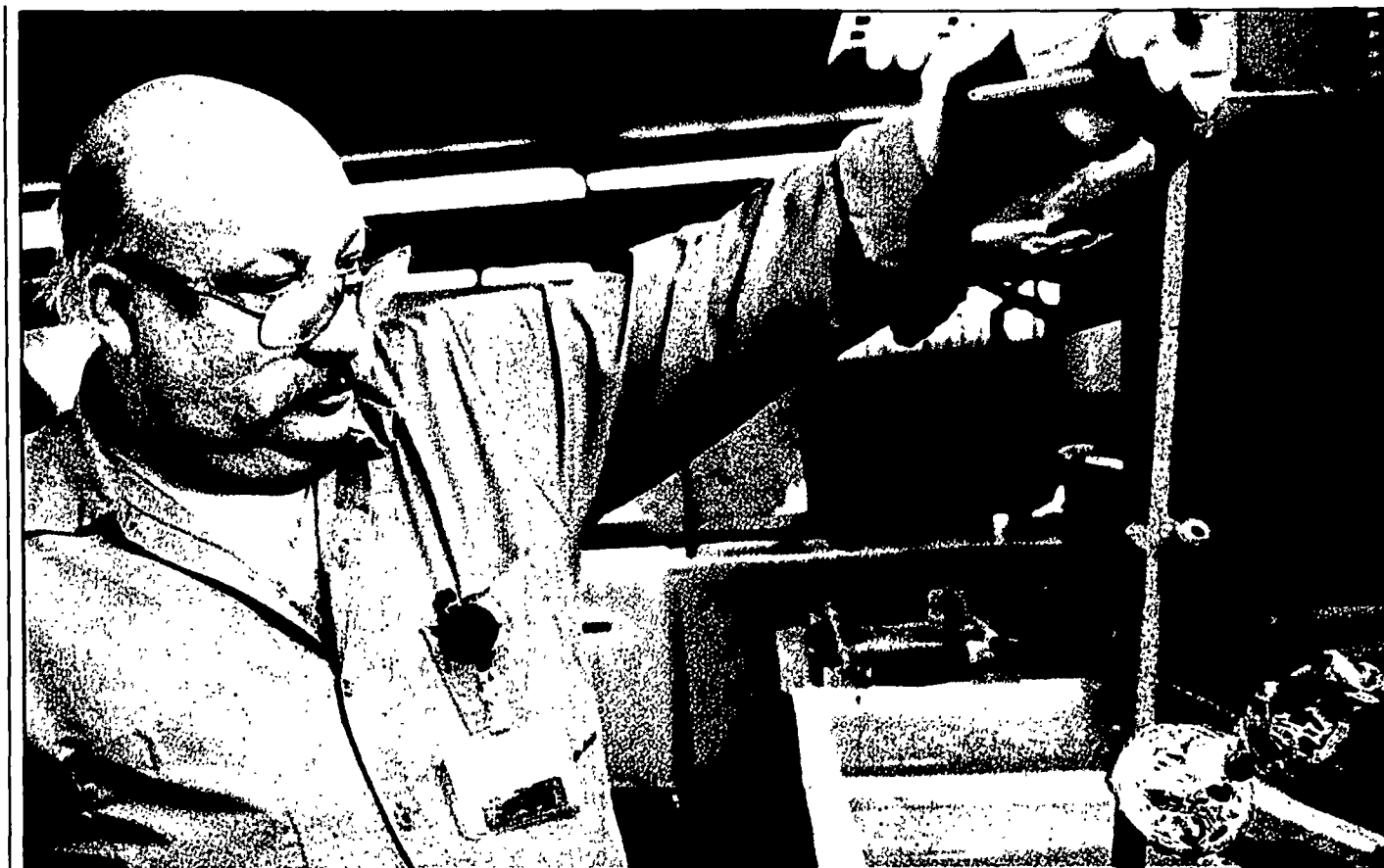
R.S. Owens & Company employee Nunzio Giganti pulls an Oscar, freshly coated in 24-karat gold, out of the tank. — Jeff Krage/For Pioneer Press
