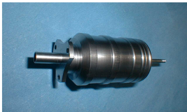
Figure 34. Evolution of the PV (dim. φ30 x 85 mm, mass 105 g) in view of possible application within a Cold Gas Micro Propulsion System
