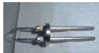
Figure 25c. Thermo-capillary LPC1, Al 2 O 3 insulator and flange
