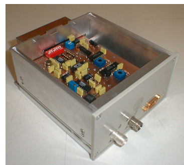
Figure 20. Electronics for the MFS (MFS-EA) integrated in the accommodation box
