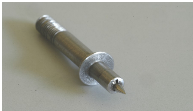
Figure 5. Titanium shutter or plunger moved by the piezo-ceramic actuation mechanism
