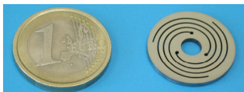
Figure 7a. Last Version of the S-shaped spring
