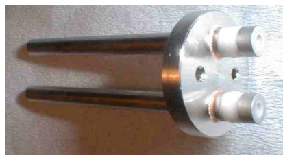
Figure 25b. Main flange and 1/8" fluid interfaces
