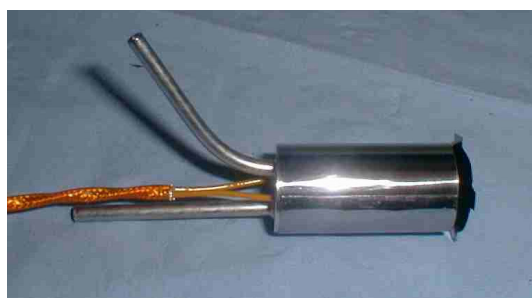
Figure 27. LPC final assembly in a cylindrical stainless steel housing
