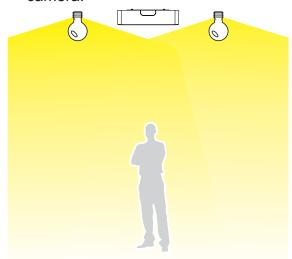
3. IMPORTANT: Make sure you measure the height of your camera. The height information is important for the accuracy of the video analytics results. Some of the other perspective information are automatically collected by the onboard G-sensor. The height information enables the horizontal and vertical keystone corrections of the field of view. Measure the distance between camera (ceiling where it is mounted) and the ground.
