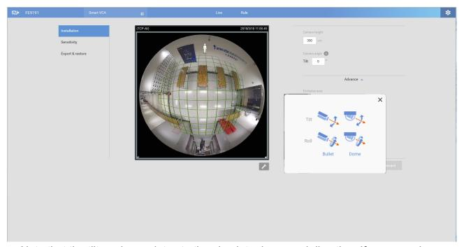
Note that the tilt angle corelates to the absolute downward direction. If a camera is installed on a ceiling, and its lens points straight downward, its tilt angle is 0 degree. If your camera lens is tilted, enter the angle related to the vertical line, e.g., 60° as shown below.
