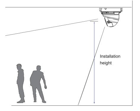
For bullet cameras or wall-mounted domes, measure the distance from the lower edge of the camera canister to the ground.
