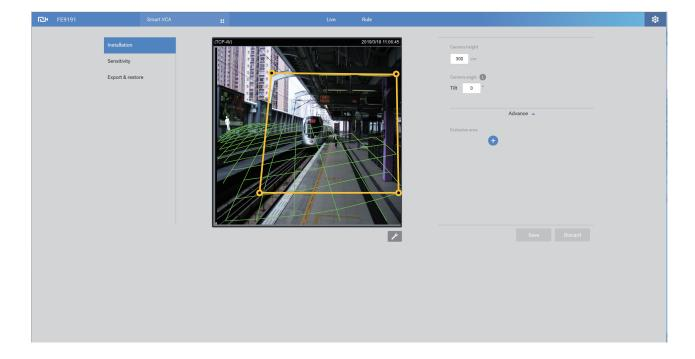
**4.** Enter the correct installation height. Please select the Auto mode for the camera to automatically acquire the shooting angles (Tilt and Roll). Users are not suggested to use the Manual mode to configure the tilt and roll angles.
