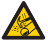
Warning for splinters. The hammer could splinter if hit against hard objects
