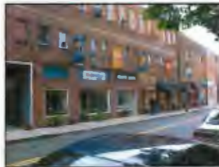
Inappropriate: block length is extremely long and the building appears too monolithic and is not adequately broken up with vertical elements.
