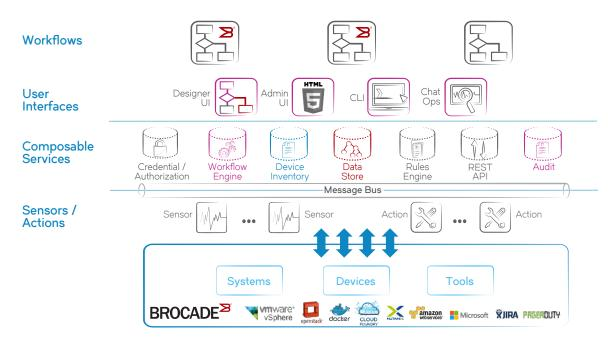
Figure 5: The Brocade Workflow Composer architecture brings workflow-centric, cross-domain network automation to IT operations.
