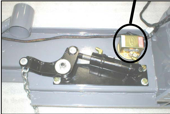
SWEEP FILTER CLOGGED SWITCH S-18 (VIEWED BEHIND BUMPER)
