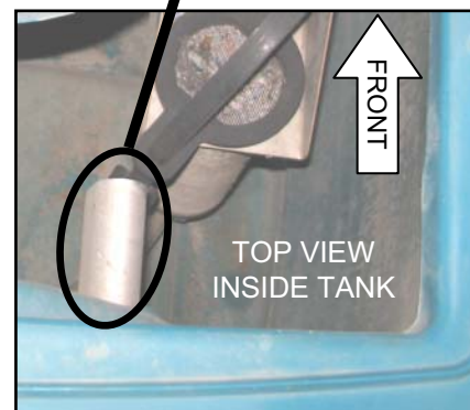
RECOVERY TANK FULL SWITCH S-15
