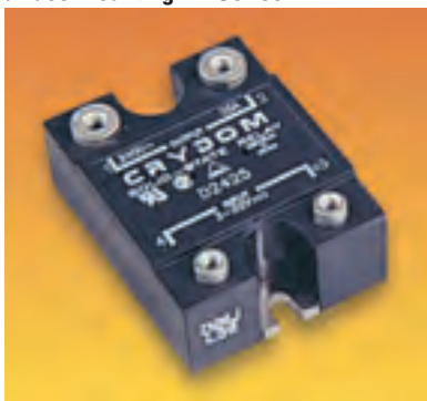
L=57.2, W=44.4, H=22.2 Fixing Centres=47.6, dia 4.4
