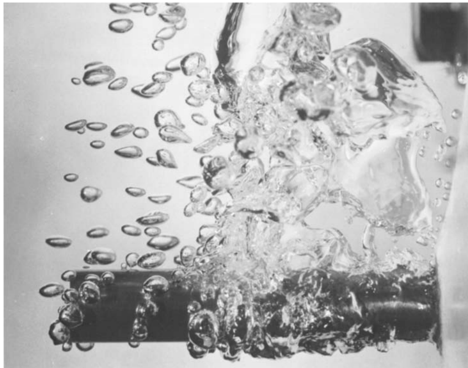
Figure 9-5 | A copper rod (6.1 mm in diameter) heated on the right side and immersed in isopropanol. Boiling regimes progress from free-convection boiling at the cooler end of the rod (left) to nucleate, transition, and finally film boiling at the right end.
