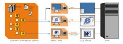
With the *Jack PC*, you can quickly and easily convert an existing enterprise LAN jack into a fully-working, remotely-managed computer without installing additional cabling. The *Jack PC* is connected at the back side through Ethernet cable to the building's LAN. The front panel is connected (through cables or wirelessly) to the display, keyboard, mouse and other peripherals.
