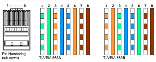
Figure 6.2 - TIA-568A and B wiring color coding
