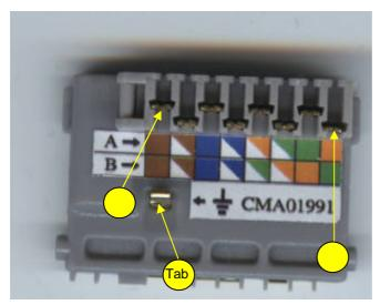
Figure 6.1 - terminal block numbering
