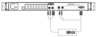
Figure 7 Connecting a B050-000 or B051-000 IP Remote Access Unit
