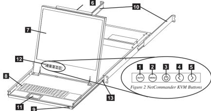
Figure 1 NetCommander KVM front panel
