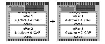
We can now activate two iCAP processor cores in nPar 1. The total number of active cores and iCAP cores in the complex has not changed but nPar 1 now has an additional two cores at its disposal.
