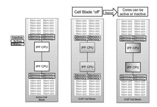
**NOTE:** On an iCAP blade with memory turned on the processors can be on or off. All active memory is available on a blade even with all cores turned off. The active memory on a blade does not depend on presence of active cores on that blade.
