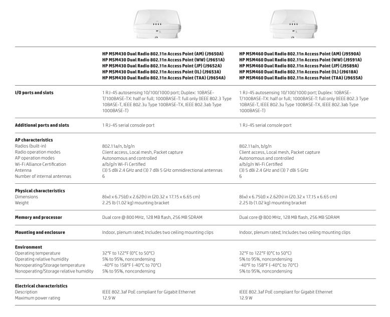
HP MSM460 Dual Radio 802.11n Access Point (AM) (J9590A) HP MSM460 Dual Radio 802.11n Access Point (WW) (J9591A) HP MSM460 Dual Radio 802.11n Access Point (JP) (J9589A) HP MSM460 Dual Radio 802.11n Access Point (IL) (J9618A) HP MSM460 Dual Radio 802.11n Access Point (TAA) (J9655A)
