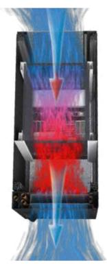
Server rack air flow with Vertiv Knürr DCL (cross-section)
