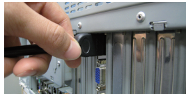
Connect an HDMI monitor
