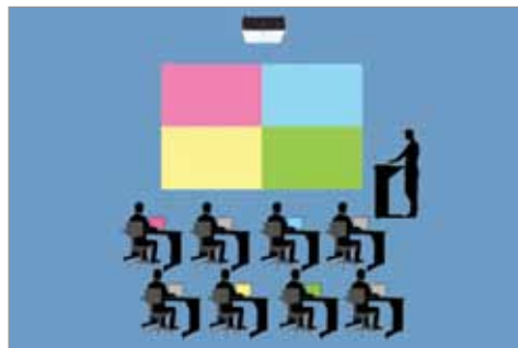
Network Multi Projection system allows for video streaming (not audio) via LAN to the projector in multiple modes.
