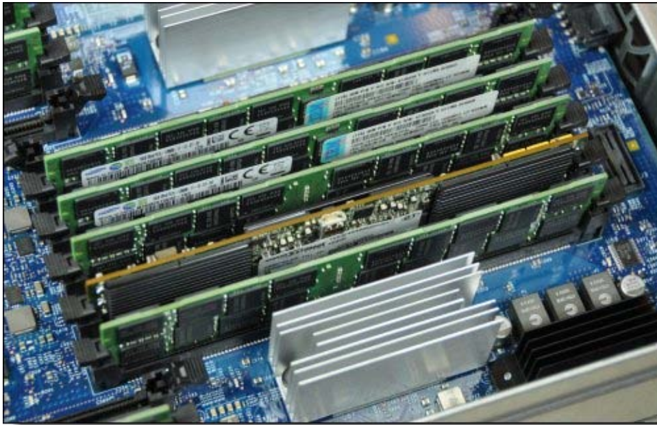
Figure 5. eXFlash DIMM installed in the Compute Book
