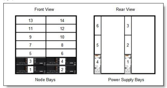
Figure 10. Power supply bay numbering
