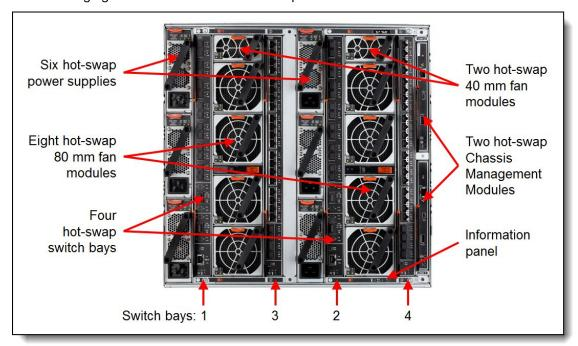
Figure 3. Rear of the Flex System Enterprise Chassis
