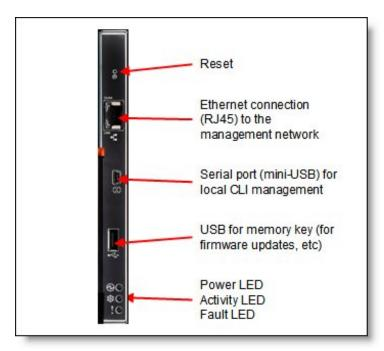
Figure 7. Chassis Management Module
