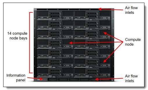
Figure 2. Front of the Flex System Enterprise Chassis
