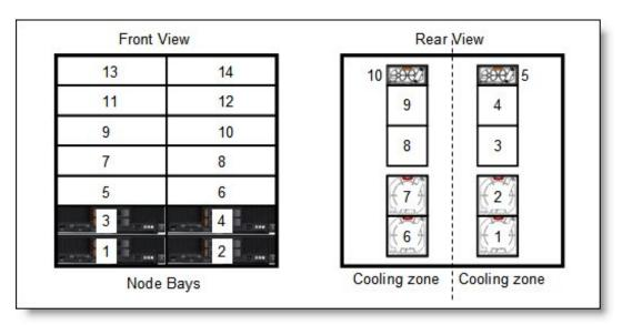
Figure 12. Fan module locations and cooling zones
