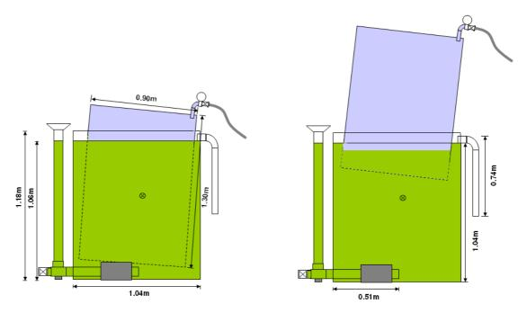
Figure 1. ARTI compact biogas plant scheme (left: with empty gasholder; right: with full gasholder) (Source: Lohri, 2009)
