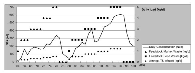
Figure 2. Varying daily feed and resulting gas production (Lohri, 2009)
