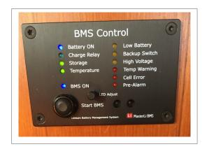
The **BMS Control** has a pre-warning system that makes it safe to utilize 93 – 95% of the lithium battery's true capacity. In event of low voltage, a three-stage Pre-Alarm with duration time of approx. 10 hours yellow LED, 27 minutes red LED and 2 minutes Buzzer.
