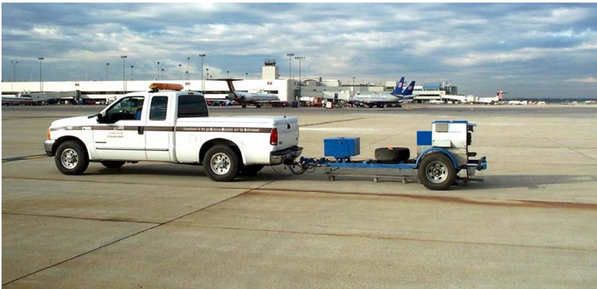
FIGURE 2.5. THE HEAVY-WEIGHT FWD POSITIONED TO PERFORM A MID-PANEL LOAD TEST
