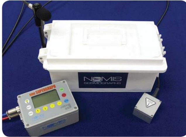
FIGURE 3.41. REMOTE SEISMOGRAPHS USED TO EVALUATE SLAB ROTATION AND LTE_{\delta} AT THE FAR ENDS OF SLABS OPPOSITE OF THE FWD LOAD LOCATION
