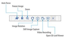
Connect the Epson ELPDC21 document camera to an EB-710Ui projector to easily capture and displays books, 3D objects and experiments. You can also add annotations directly to a projected live image without the need of a PC. To simplify the process you can operate the document camera from the toolbar on the projection screen.
