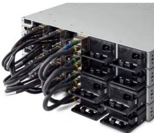
Figure 4. Cisco Catalyst 9300 Series StackPower
