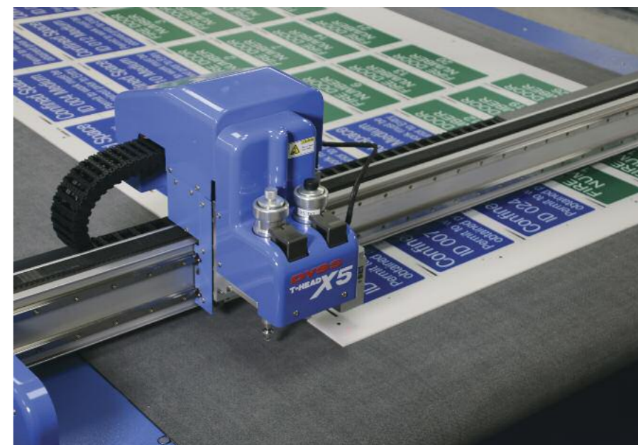
K-Cut Vision System on DYSS X5 locating position of printed sheet.
