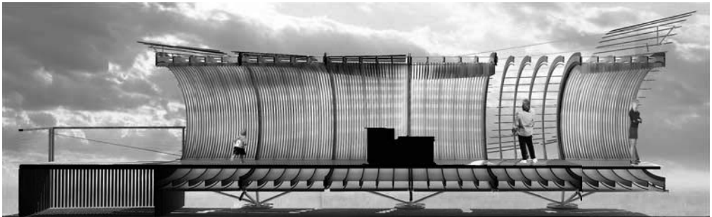
Figure 5: Exterior view of early Design Development phase multilayered envelope with doubly curved shell
