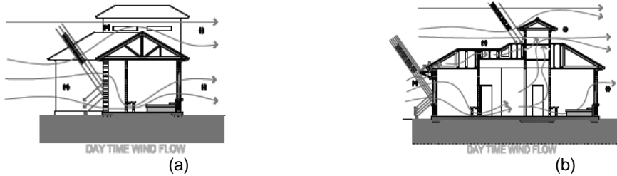
Figure 7: Wind flow during day time through: a) Optimized Haitian house Option-1 and b) Optimized Haitian house Option-2. Source: (Authors 2013)
