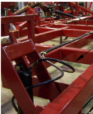
ROUTE HOSES BEHIND TOWER
