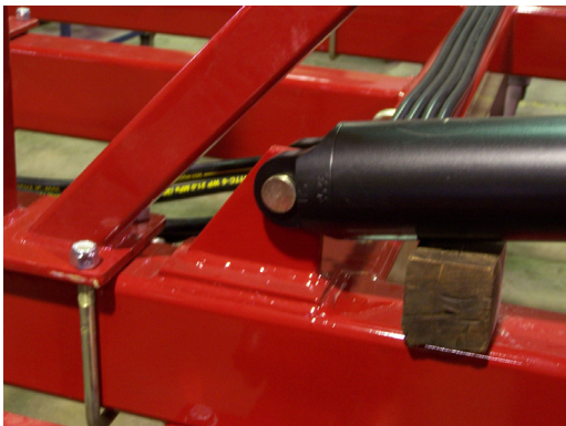
Fig 1. When charging the circuit, prop up cylinder with block of wood. Be sure the rod can extend freely without striking anything.
