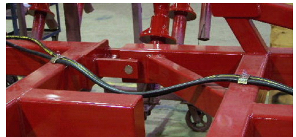
LEAVE A 7-10cm DROOP OF HOSE AT WING HINGES
