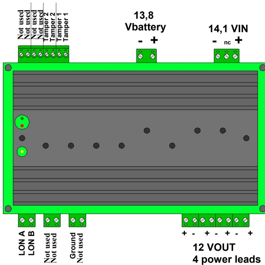
Figure 5. Cable Connections
