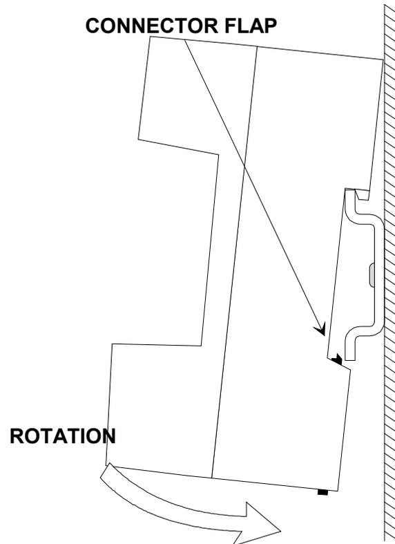
*Figure 11 – Mounting on the DIN Bar*
