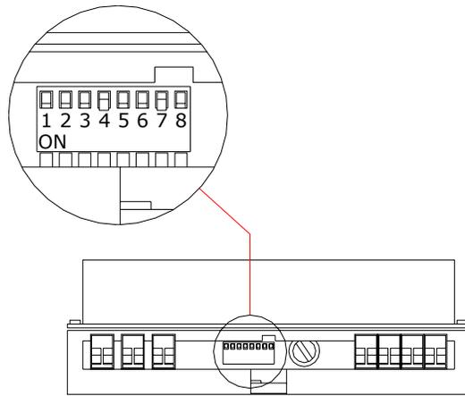
*Figure 3: DIP Switch – Setting the battery recharge*
