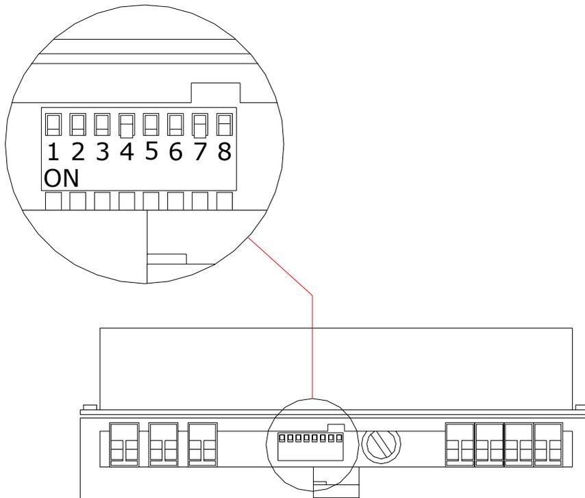
*Figure 4. DIP Switches – setting the output current*
